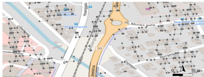
**Fig. 2.** Example of graphs generated from InSAR-based ground-movement maps. Each node represents a pixel in the EGMS dataset for a small urban area.
